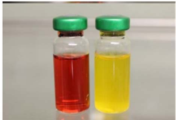
Acid Producing Bacteria (APB) Serial Dilution
