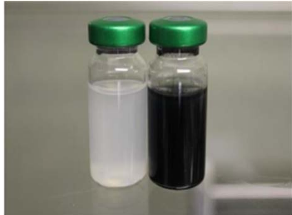
Sulfate Reducing Bacterial (SRB) Serial Dilution
